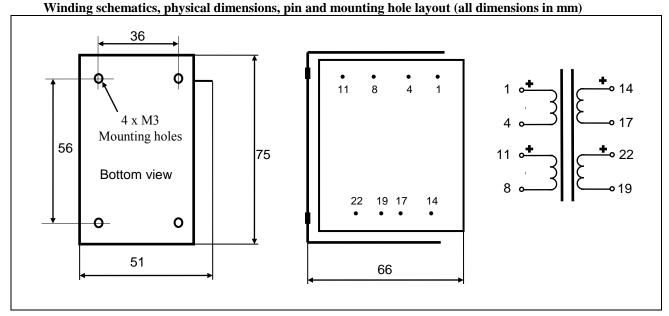
Weight: 0.75 kgStatic resistance of each primary: 560 Ω Static resistance of secondary:  $560 \Omega$ Isolation between windings / between windings and core: 4 kV / 2 kV Max recommended DC current through primary windings: 50mA (3W heat dissipation)
